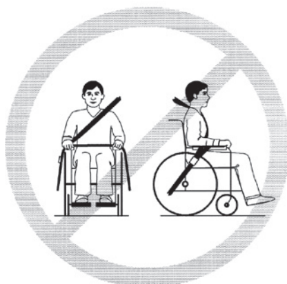
Figure 4: Belt restraints should not be held away from the body by wheelchair components or parts, such as the wheelchair armrests or wheels.
