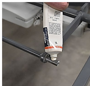
Apply grease on axle
