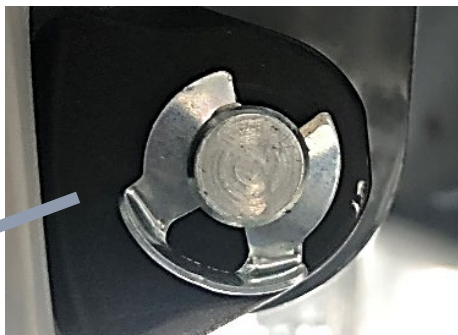
Retaining clip in the other end
