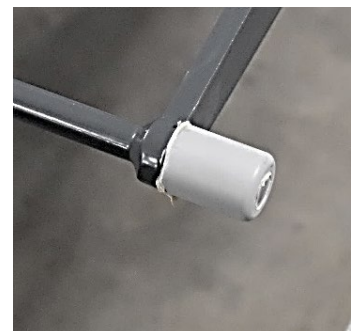
Remount wheel runners on axle
