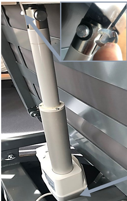
Location of retaining clip and bolt
